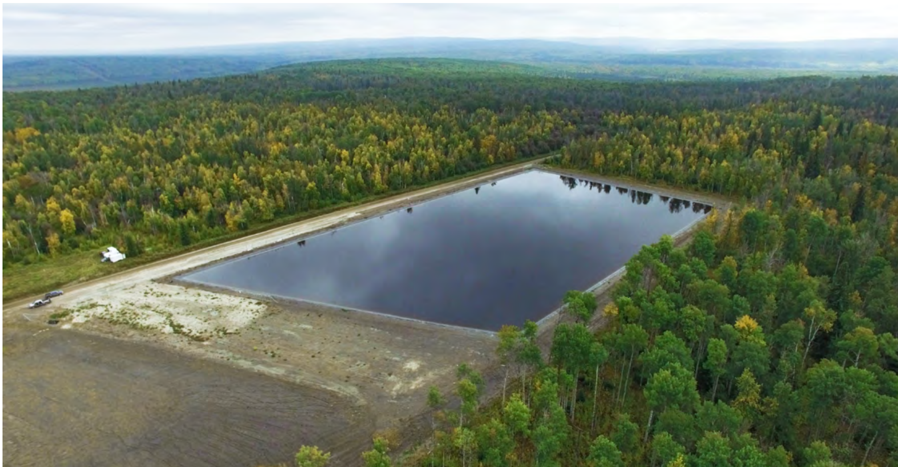
Birchcliff's 10-27 water storage reservoir stores 135,000 m 3 of fresh water transferred from multiple sources during spring freshet.
